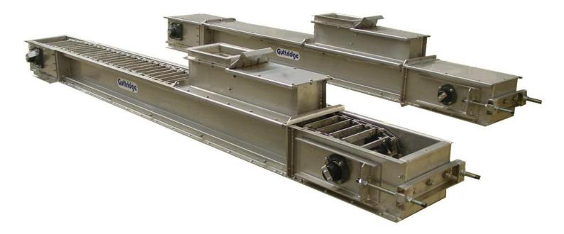
Chain & Flight Conveyors are an essential part of many conveying and storage systems dealing with powdered, granular, flaked or pelletised materials. Being simple and robust in design and easily maintained, they provide low cost efficient handling equipment with many applications in manufacturing and processing factories.
