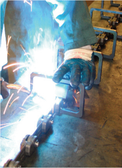
The chain and flight configuration is designed and fabricated to suit the application
