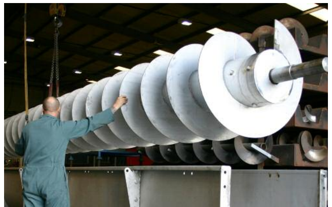
A large heavy duty screw conveyor for handling sugar.
